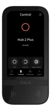
KeyPad TouchScreen can arm and disarm the entire object or specific groups, and activate **Night Mode**. Use the **Control** tab to change the security mode. You can control the security using KeyPad TouchScreen through:
