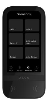
The separate keypad tab holds up to six buttons that control one <u>automation</u> <u>device</u> or a group of devices. Group scenarios provide more convenient control over multiple switches, relays, or sockets simultaneously.
