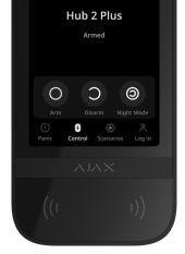
If Group Mode is enabled, users see the security mode of each group separately. The group is armed if its button outline is white and it is marked with  $\bigcirc$  icon. The group is disarmed if its button outline is grey and it is marked with  $\bigcirc$  icon.
