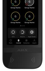
KeyPad TouchScreen can participate in two-stage arming but cannot be used as a second-stage device. The two-stage arming process using Tag, Pass or smartphone is similar to using a personal or general code on the keypad.
