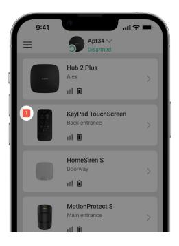
When a KeyPad TouchScreen malfunction is detected, the Ajax app displays a malfunction counter on the device icon. All malfunctions are indicated in the keypad's states. Fields with malfunctions will be highlighted in red.
